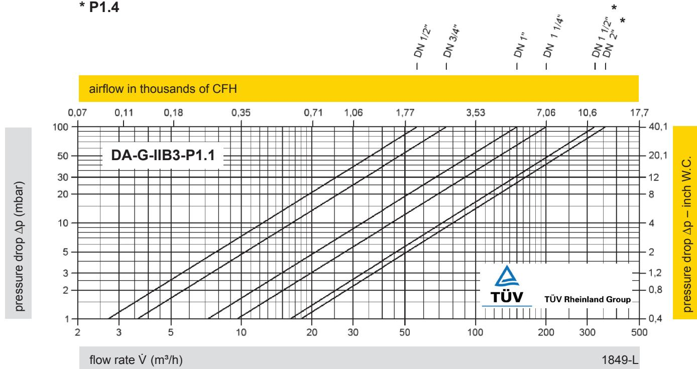
The flow capacity charts have been determined with a calibrated and TÜV certified flow capacity test rig. Volume flow  $\dot{V}$  in ( $\text{m}^3/\text{h}$ ) and CFH refer to the standard reference conditions of air ISO 6358 (20°C, 1bar). Conversion to other densities and temperatures refer to Vol. 1: "Technical Fundamentals".
