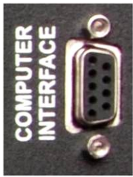
d) Communication (fuse D-Sub 9-jack)
