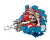
All NP pump models feature Blackmer's revolutionary sliding-vane operating principles, which guarantee consistent volumetric performance, even after significant in-service time. This eliminates the efficiency-robbing "slip" that shortens lobe and gear pump life, and improves production yields by stripping lines of residual product. NP pumps also offer excellent self-priming and dry-run capabilities.
