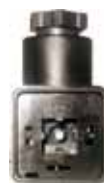
1578501 Quick connection connector DIN 43650, suitable for all IM2 coils. Cable gland Pg9 (cable diameter 6 \div 8 mm). Adjustable cable outlet in 4 positions every 90^{\circ} .
