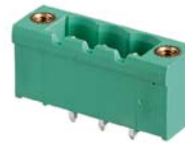
pitch 5/5.08 mm straight version locking screw flange
