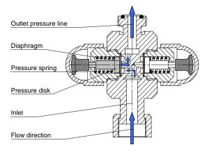
If the admission pressure increases beyond the opening pressure, the diaphragm is raised against the spring force and the valve opens.
