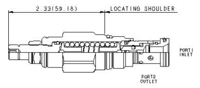
Direct-acting relief cartridges are normally closed, pressure-limiting valves used to protect hydraulic components from pressure transients. When the pressure at the inlet (port 1) reaches the valve setting, the valve starts to open to tank (port 2), throttling flow to limit the pressure rise. These valves are smooth and quiet, essentially zero leak, \_ dirt tolerant, immune to silting and are very fast.
