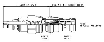
Pilot-operated, pressure reducing/relieving valves reduce a high primary pressure at the inlet (port 2) to a constant reduced pressure at port 1, with a full-flow relief function from port 1 to tank (port 3).
