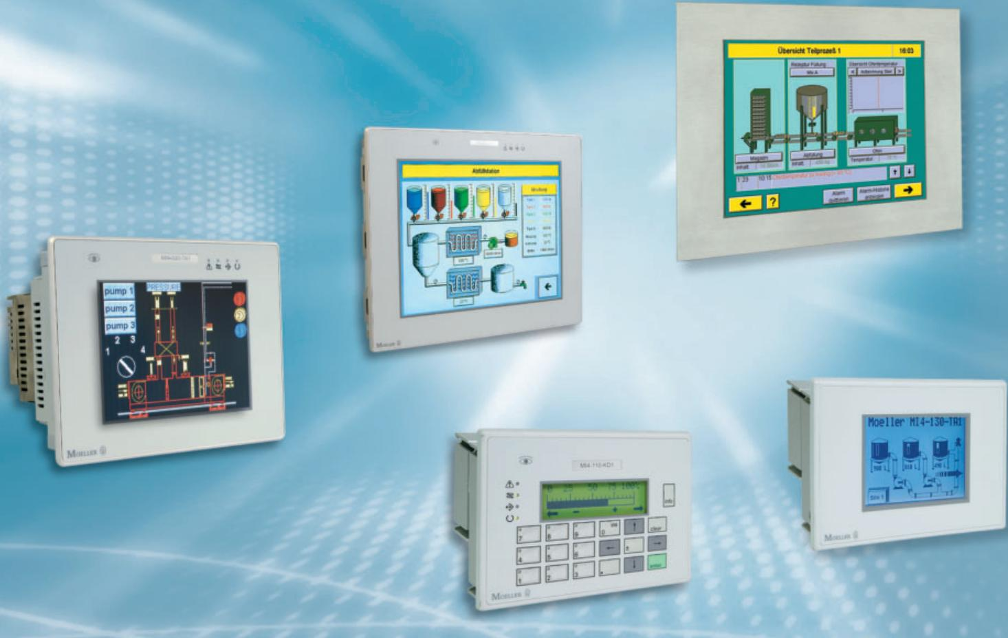
With its MI4 and MV4 operator and display units, Moeller offers you a product range for Man/machine communication that allows you to implement solutions quickly and in the optimum fashion. The offering includes units from graphics-capable Text Operator panels with 4 x 20 characters and 11 keys, up to 15" TFT Touch Operator panels with a resolution of 1024 x 768 pixels.
