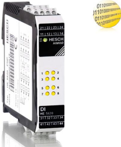
The digital input module HE 5820 acquires up to eight binary signals from the process level and transmits these to the higher-level bus system. The communication with the field bus coupler takes place over an asynchronous serial RS-485 connection. In the event of service, the module can be exchanged quickly and without complications in running operation (Hot Swap). The module supplies a power supply per input of 24 V DC with a maximum current of 25 mA for the direct connection of e.g. proximity-
