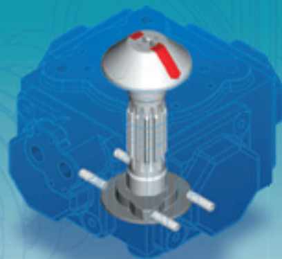
Limit stop for open-close and intermediate positions
