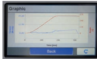
Graphic display of screwdriving graphs
