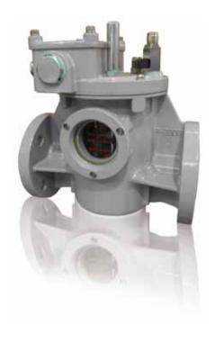
The relay for OLTC application is positioned in the pipe work between the on-load tap-changer head and the oil conservator. This relay responds only if oil flow occurs from the on-load tap-changer head to the oil conservator. If this happens, the flow vane switches the reed . The circuit breakers are tripped and the transformer is de-energized.
