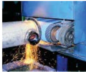
API's additional grinding process flattens tube ends and tubesheets which reduces risk of crevice corrosion, ensures even gasket compression and eliminates cracking of casting during manufacturing and servicing of units.
