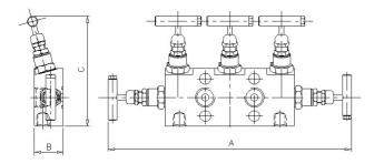
The 'Y53' Type 5 valve manifolds are designed for direct mounting to differential pressure transmitters, with separate isolation and vent for LP and HP inlets plus equalising valve for simple calibration. Each needle valve head is designed for safe and reliable isolation, giving bubble tight shut off, with non-rotating & anti-galling tip and dynamic self-adjusting spindle seal to give long service life in a variety of service conditions.
