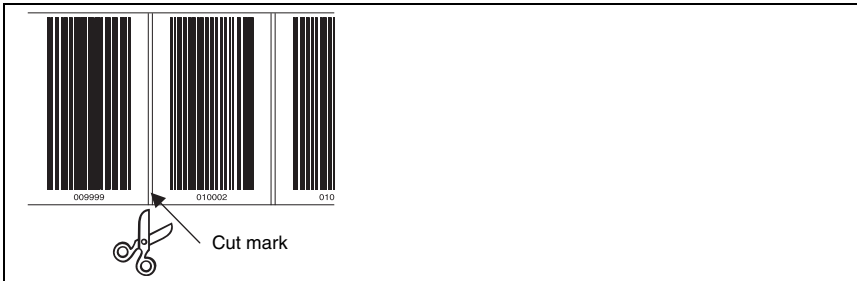
Figure 6.3: Cut mark on the barcode tape
