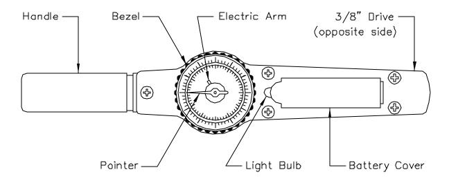
Note: For consistency and accuracy it is suggested that this torque tool be dedicated for use in one direction only. Should this not be practical for your application the following procedure should be followed for initial setting or when changing direction. It is recommended that the tool be operated 3 or 4 times at half load in the torque direction that will be used. Full load may now be applied for your application.
