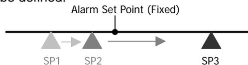
3.4.2.1 Absolute Upper Limit Alarm (Alarm Code 05, Alarm release in the first alarming situation)
