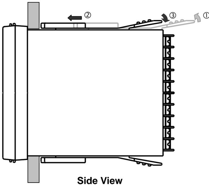
1 - Put the mounting bracket in the rail on the top & bottom of the case.
