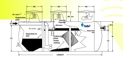
T1: INLET S: SETTLING CHAMBER A: OIL STORAGE CHAMBER B: SEPARATING AREA K: COALESCING PLATES M: MANHOLES T2: OUTLET Ø: DIAMETER L: LENGTH
