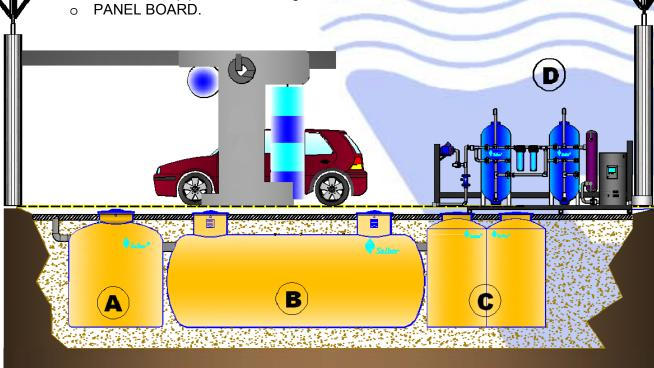
A: Solids settling tank. B: Hydrocarbon separator C: Lung tank and accumulator. D: Reuse station
