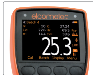
The gauge updates and displays the statistical values as each individual reading is taken
